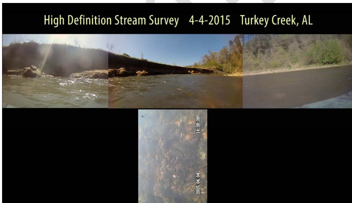
Figure 12: An example of the video from the kayak HDSS in a poor quality section of Turkey Creek. Note the bank failure on the left side of the image.
